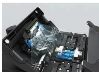
3 LED's provide a bright operation environment
